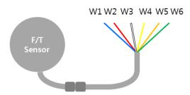
Open-end of the Robot Cable (high flex)
